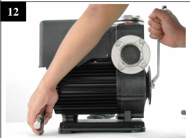
Using wrench to tighten up the lock nut. ※Torque 220 kgf · cm
