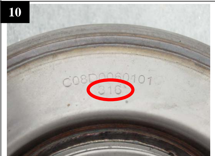
Identify mark 316 on the intermediate chamber.
