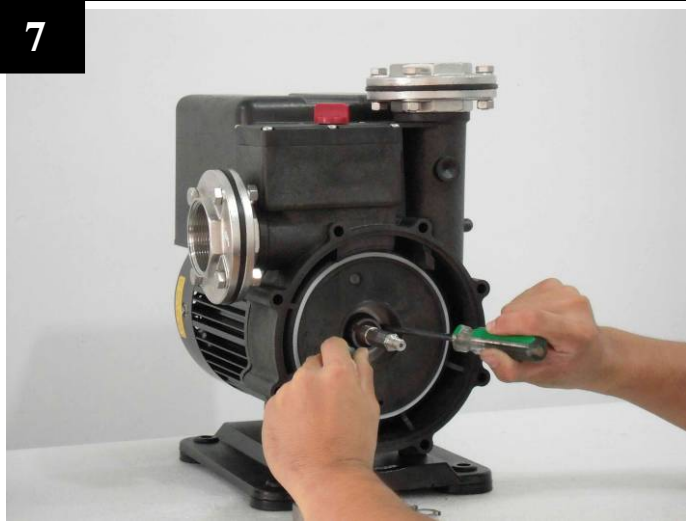
Remove the rotary parts of mechanical seal.
