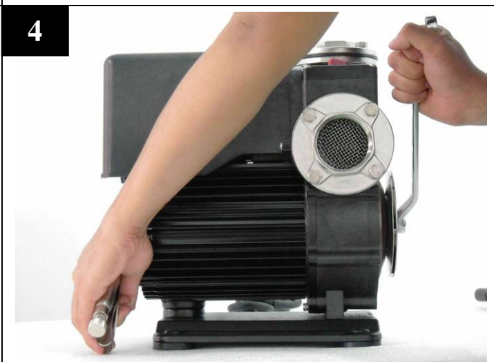
Using wrench to loose the lock nut.
