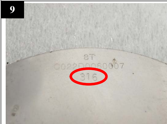
Identify mark 316 on the impellers.
