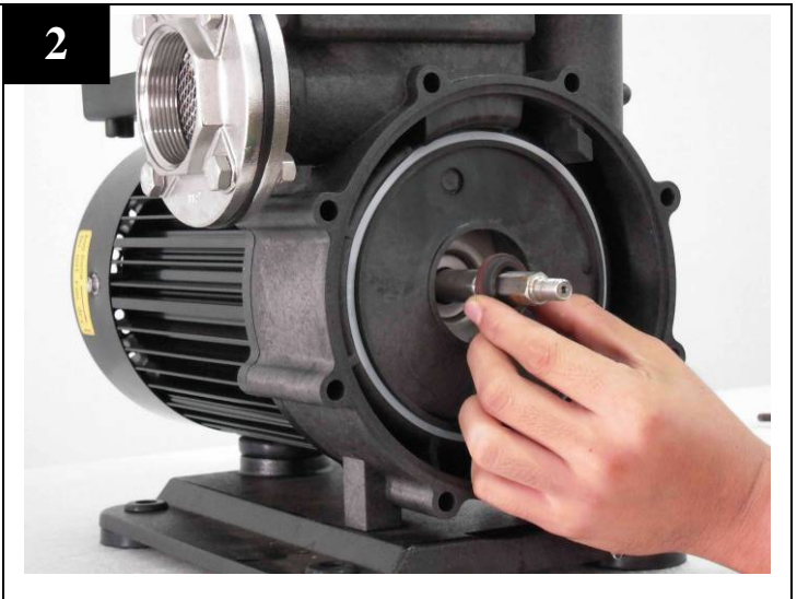
2 Place the stationary parts in position.
