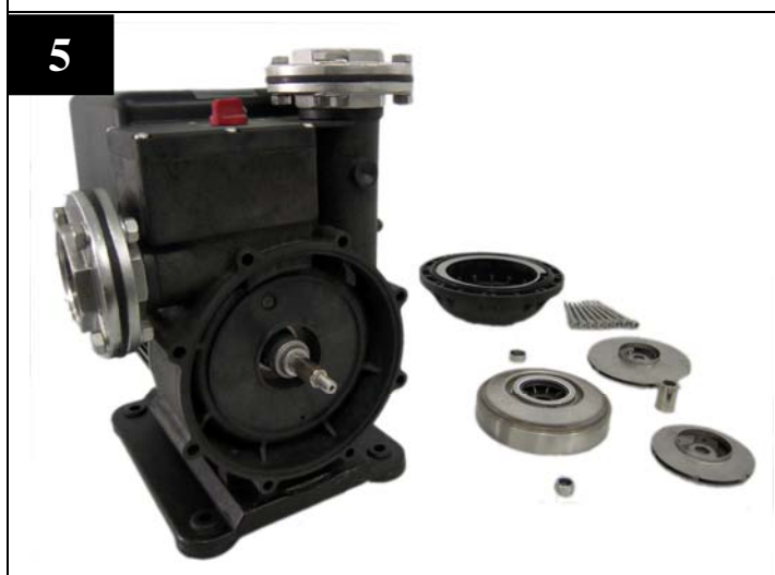
Remove all impellers, sleeves and intermediate chamber and place them in order.
