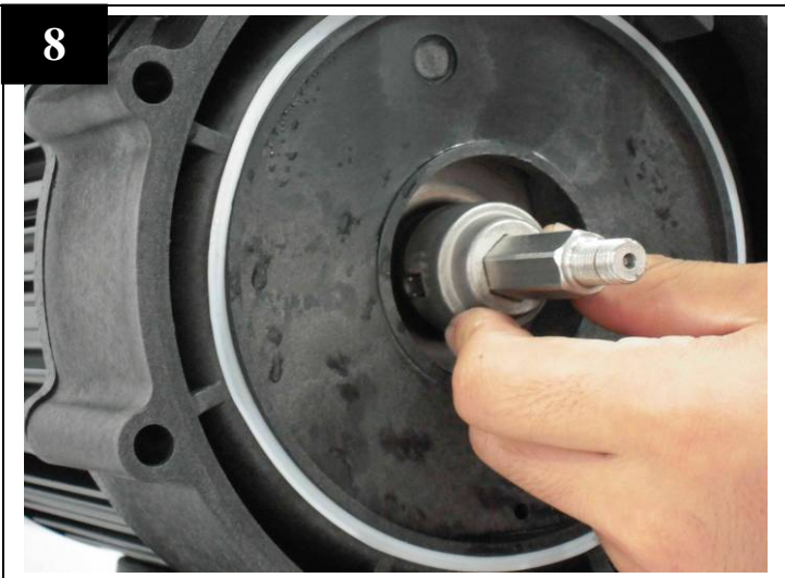
Place the cap onto rotary parts.
