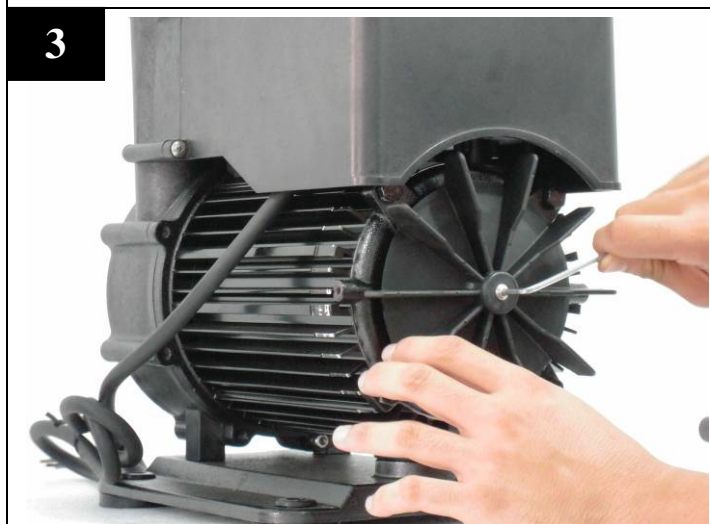
Using Allen wrench to remove the motor fan.
