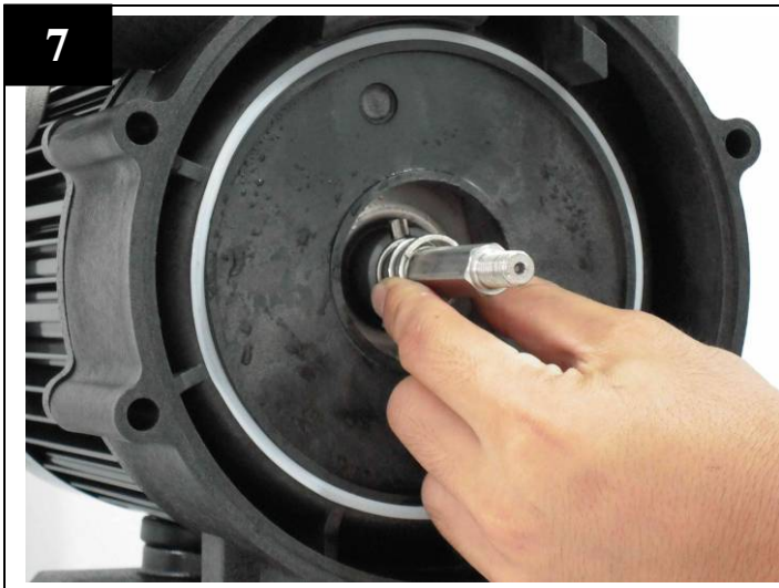
Place the spring onto rotary parts.
