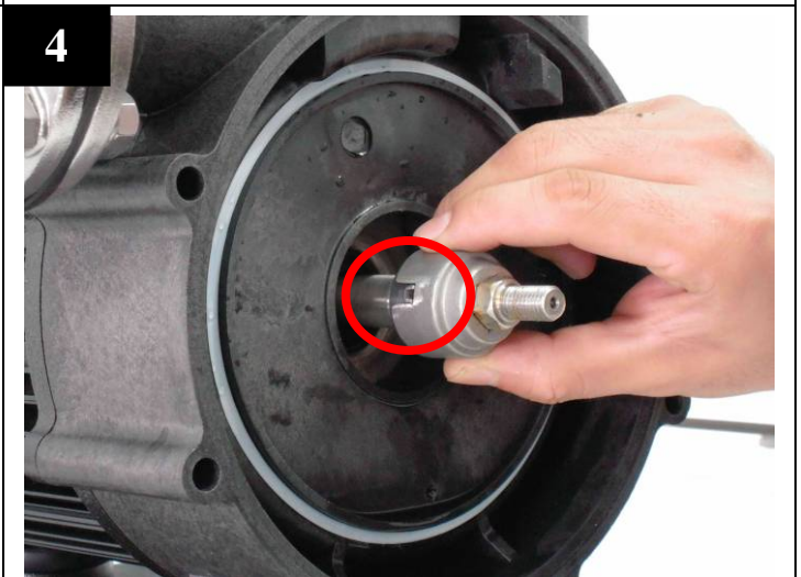
4 Before press in rotary parts, insert the sleeve through the hex shaft aligning the slots on sleeve to tabs on washer.
