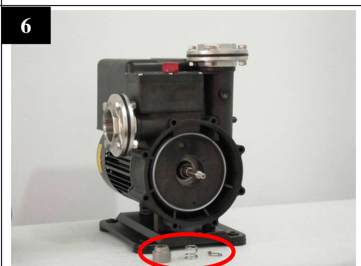
Remove the cap, spring and washer.
