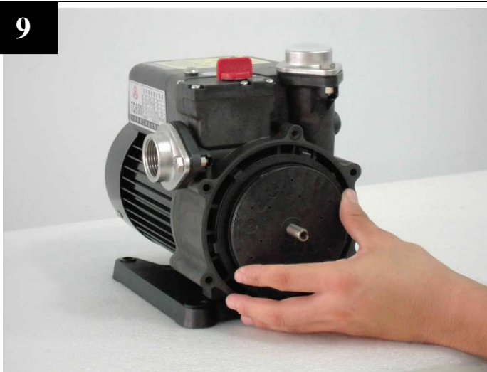
Assemble the 2nd stage impeller.
