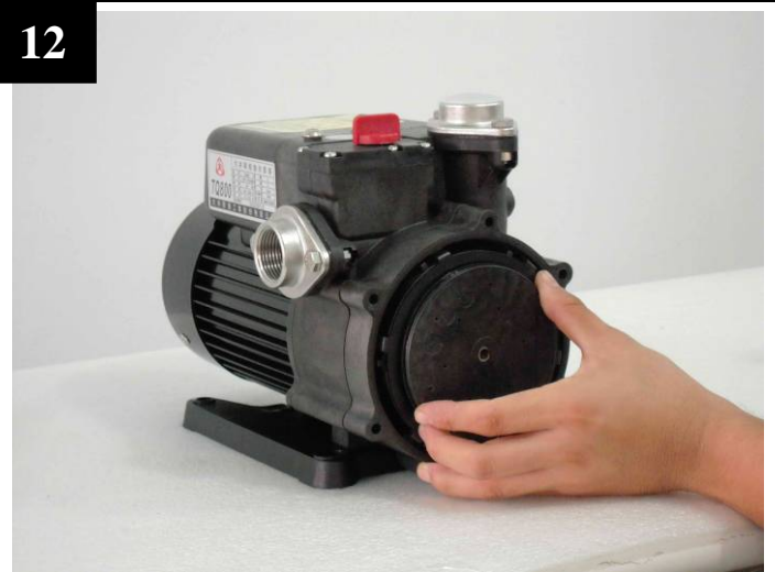
Install the 3 rd stage impeller. (Disregard the process for TQ400)
