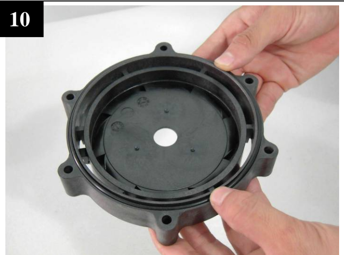
Install O-ring onto the intermediate chamber seat. (Disregard the process for TQ400)
