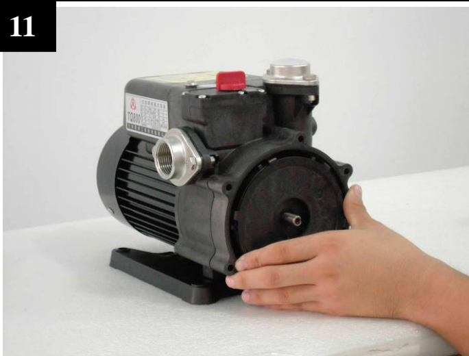
Install intermediate chamber and chamber seat. (Disregard the process for TQ400)
