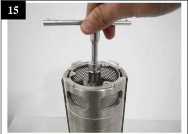
Rotate the shaft and make sure no rubbing noise inside. Otherwise, loose the screws and repeat the above process until the rotation is smooth.
