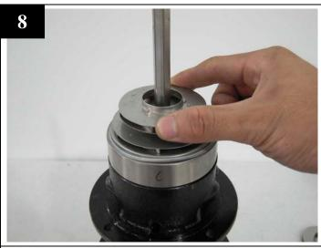
Place back all impellers, sleeves and intermediate chambers in order.
