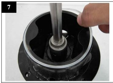
Place a new gasket on pump casing.
