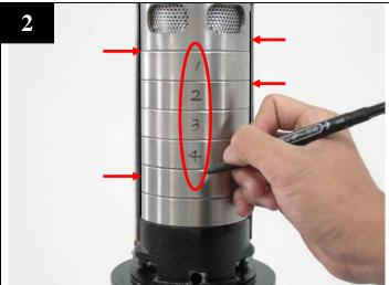
Mark the number of the intermediate chambers and draw a line along with straps.
