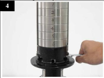
Loose the nuts on straps. Remove the 2 straps.
