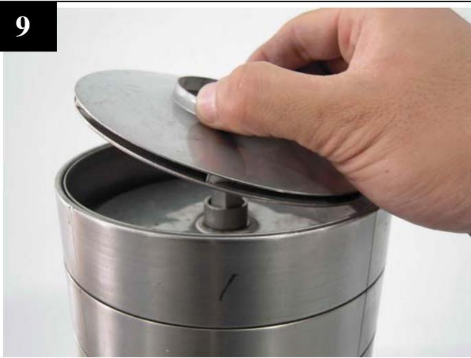
Remove all impellers, sleeves and intermediate chambers.
