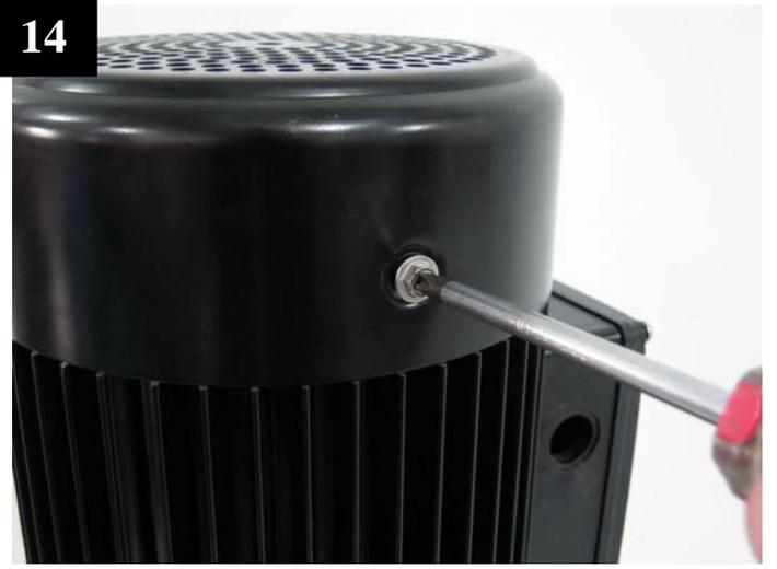
Install the motor fan cover.
