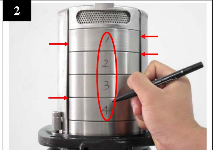
Mark the number of the intermediate chambers and draw a line along with straps.
