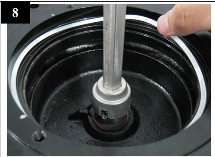
Place a new gasket on pump casing.
