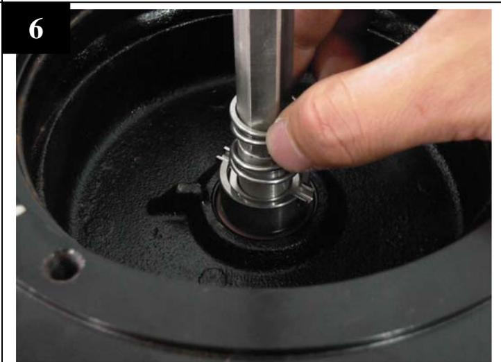
6 Place the spring onto rotary parts.
