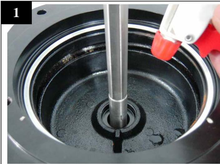
1 Spray water on the shaft as lubrication.
