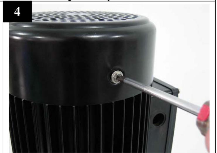
Loose the screws and remove the motor fan cover.
