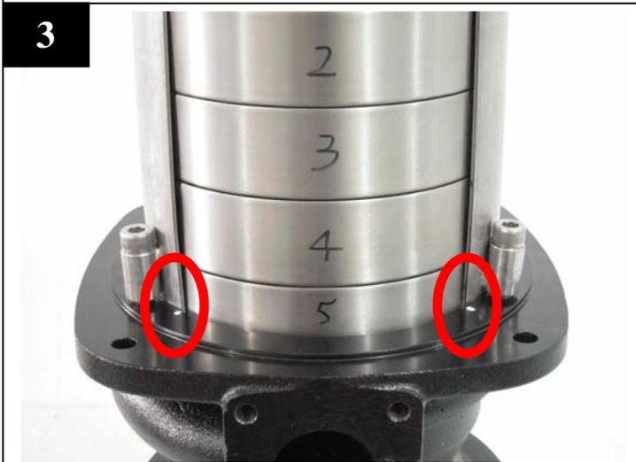
Draw the line all the way down to pump casing.
