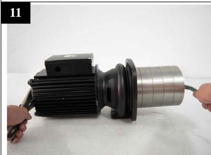
Using wrench to tighten up the lock nut.
