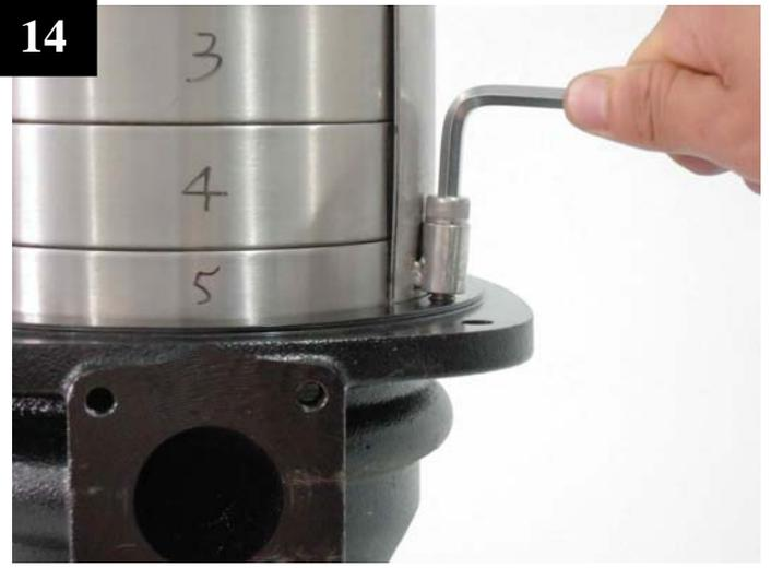
Tighten up the nuts on straps.
