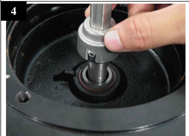
4 Before press in rotary parts, insert the sleeve through the hex shaft aligning the slots on sleeve to tabs on washer.
