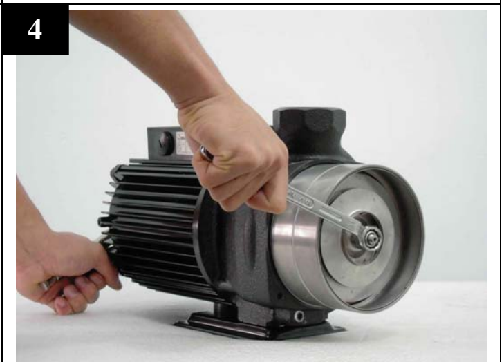
Using wrench to loose the lock nut.
