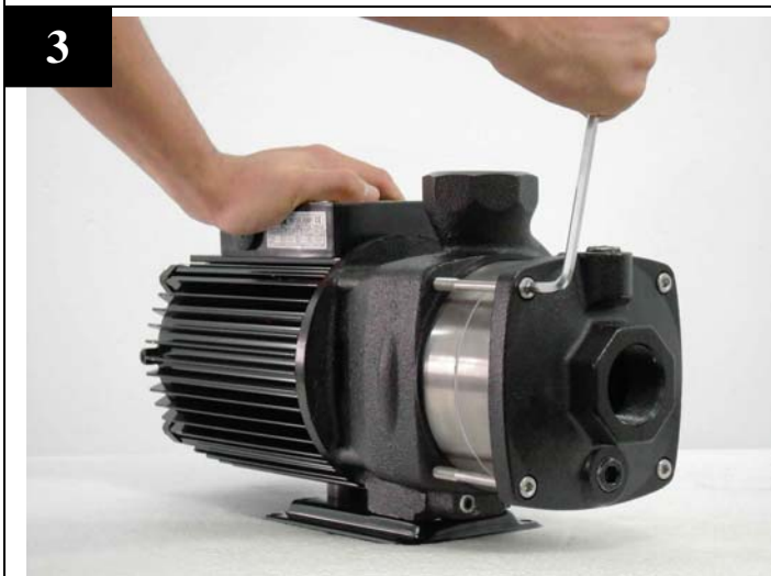
Using Allen wrench (metric size) to loose the stud bolts and remove pump cap.
