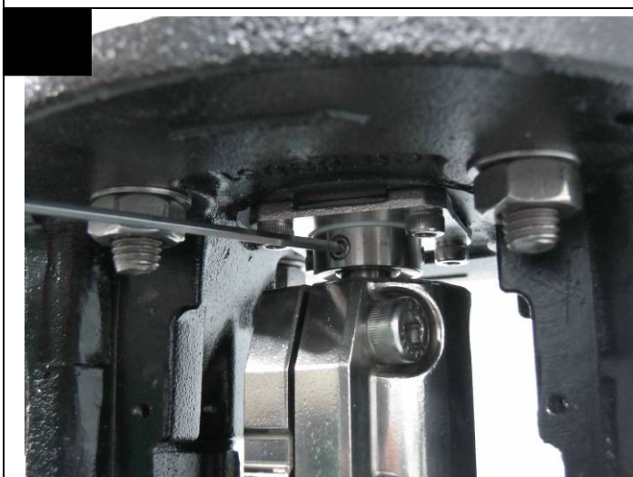
Tighten up the stud bolts on mechanical seal. ※torque 45 kgf · cm
