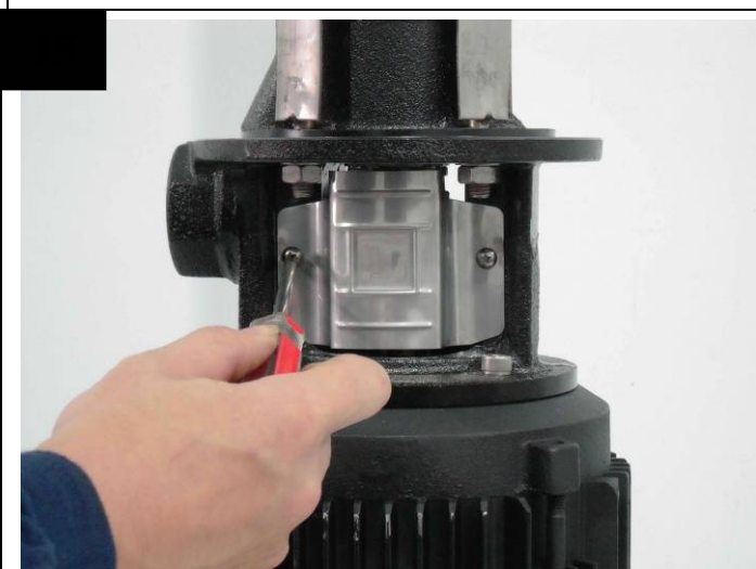
Install the coupling cover. ※torque 20 kgf · cm
