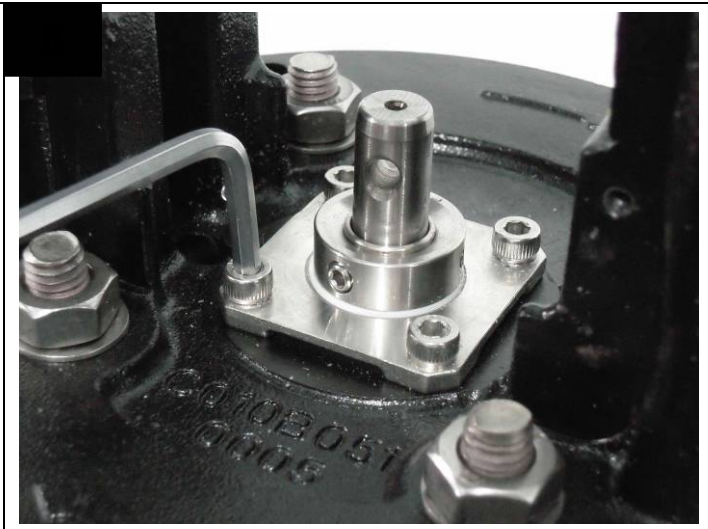
Loose the stud bolts (#4 Allen wrench) on the mechanical seal.
