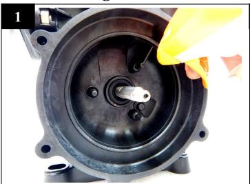
Spray water on the shaft as lubrication.
