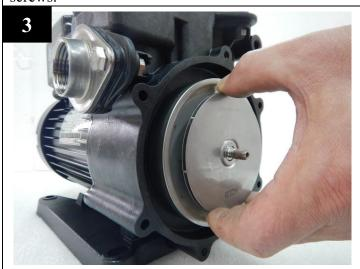
Remove all impellers, sleeves and intermediate chambers.
