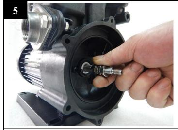
Remove the rotary parts of mechanical seal.
