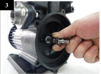
Put on the rotary part of mechanical seal.
