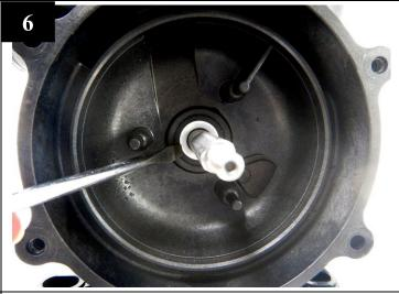
Remove ceramic parts from mech seal kit.
