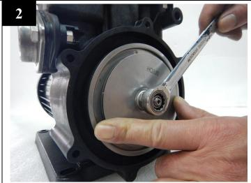
Using wrench to remove the stud bolt.
