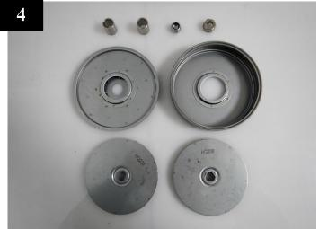
place all impellers, sleeves and intermediate chambers in order.
