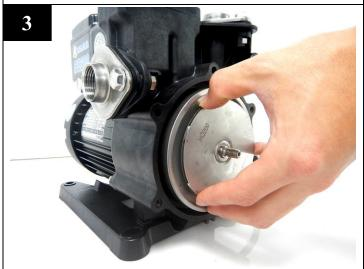
Remove all impellers, sleeves and intermediate chambers.
