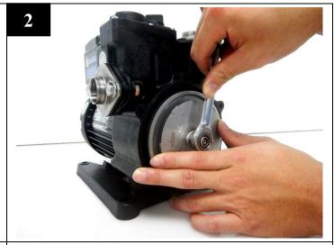
Using wrench to remove the stud bolt.
