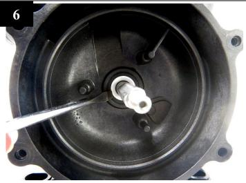
Remove ceramic parts from mech seal kit.
