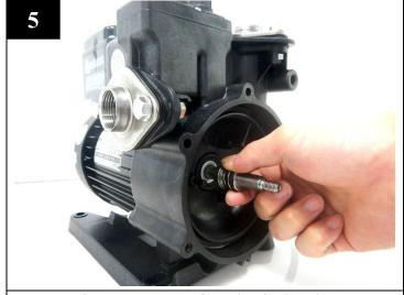
Remove the rotary parts of mechanical seal.
