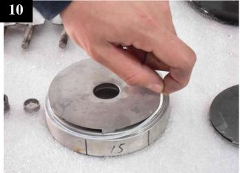
Remove the gasket from the inter-mediate chambers.
