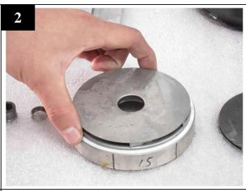
Please new gasket on inter-mediate chambers (only the stages close to pump end installed with gasket)
