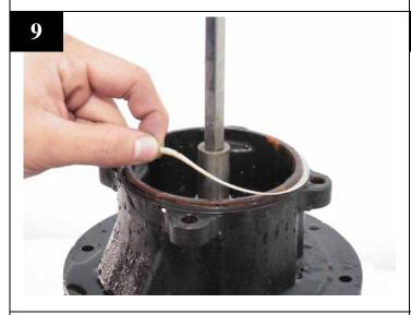
Remove the gasket from the pump casing.
