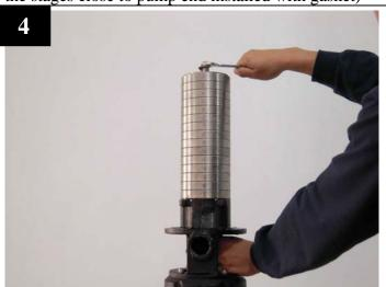
Hold the coupling and tighten up the lock nut.
