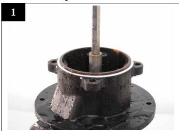
Place a new gasket on pump casing.
