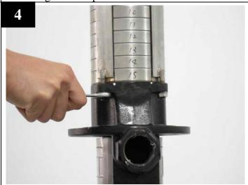
Loose the screws on stacked stages
