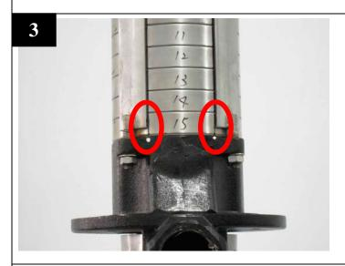
Draw the line all the way down to pump casing.
