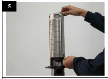
Remove the 4 straps and suction inter-connector
