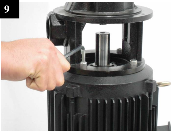
Loose the screws (#6 Allen wrench) on the motor.
