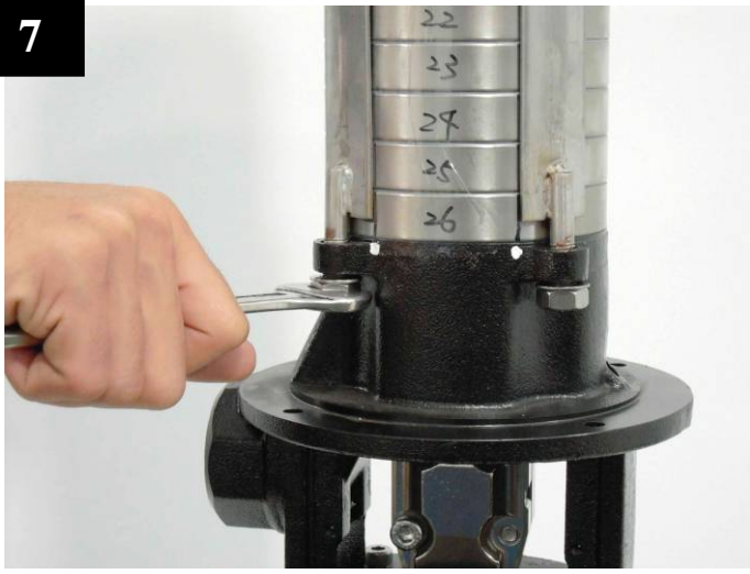
Loose the Hex. nuts (#17 metric wrench) on the coupling
