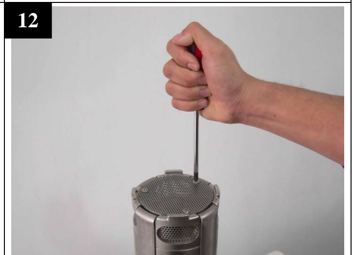
Tighten up the strainer. ※torque 30 kgf · cm
