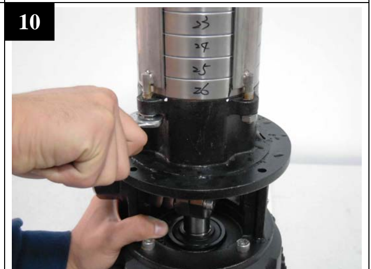
Tighten up the screws on the motor. ※torque 180 kgf · cm
