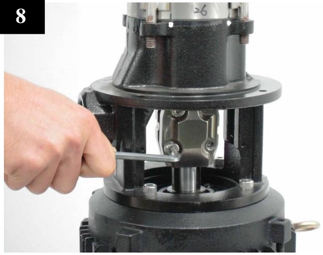
Remove the coupling (#6 metric Allen wrench)
