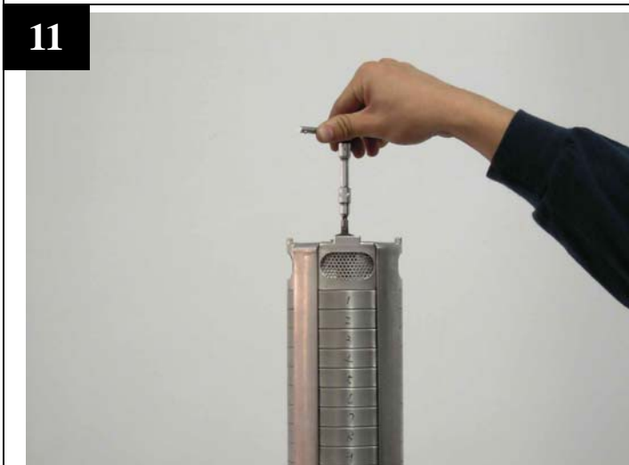
Rotate the shaft and make sure no rubbing noise inside. Otherwise, loose the screws and repeat the above process until the rotation is smooth.
