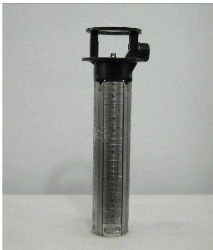
Place the pump end on work bench and remove the hex nuts.
