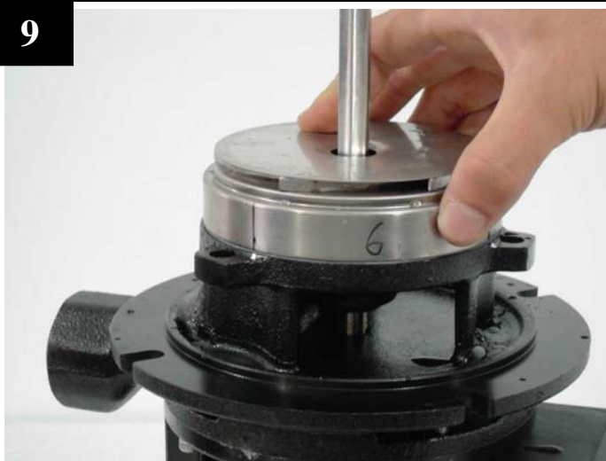
Remove all impellers, sleeves and intermediate chambers.
