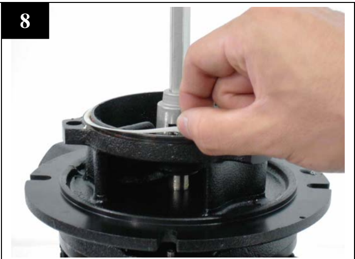
Place a new gasket on pump casing.
