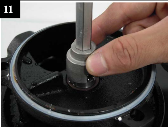
Remove all impellers, sleeves and intermediate chambers.
