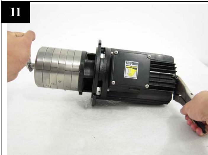
Using wrench to tighten up the lock nut. ※torque 140 kgf · cm
