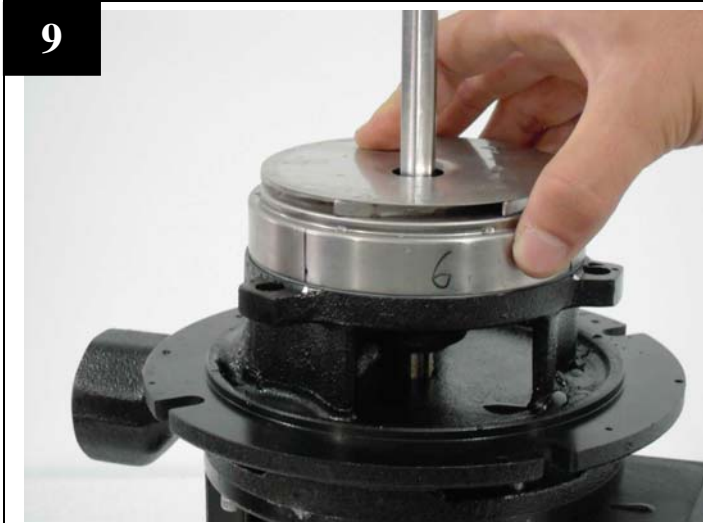
Place back all impellers, sleeves and intermediate chambers in order.
