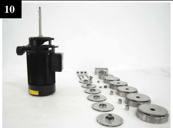
place all impellers, sleeves and intermediate chambers in order.
