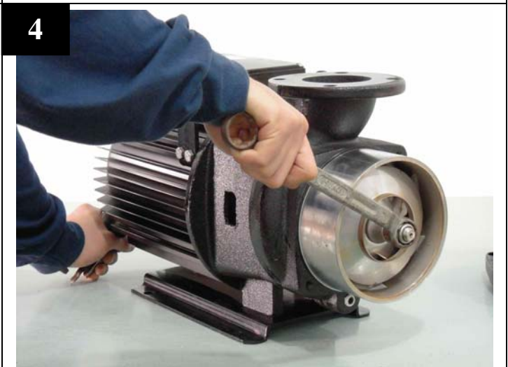
Using wrench to loose the lock nut.
