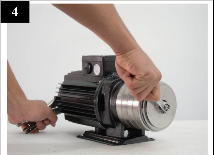
Using wrench to loose the lock nut.
